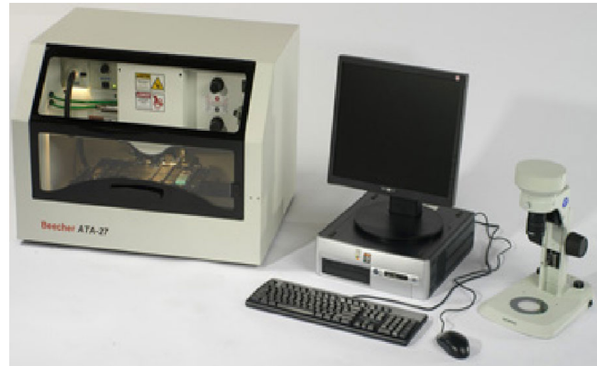
Fig. ATA-27 TMA, from Beecher with a transfer capacity of 26 cores from different donor blocks to each recipient block.
